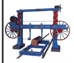
Built of double channel pillars and heavy duty frames accurately planned and polished with Joint Slide (brass patty) for smooth up and down. The saw wheels mechanically balanced are mounted on taper roller bearing in dust proof housings. Also fitted with tow saw guides of steel.the jack screw is fitted with thrust bearing With Log Holding Blocks with vices, also available with Automatic Raising And Lowering Arrangement on Order.
